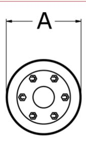
A = 208 D1 = 60 D2 = 90 L = 206 Nom. torque NM (Tkn) = 5000
